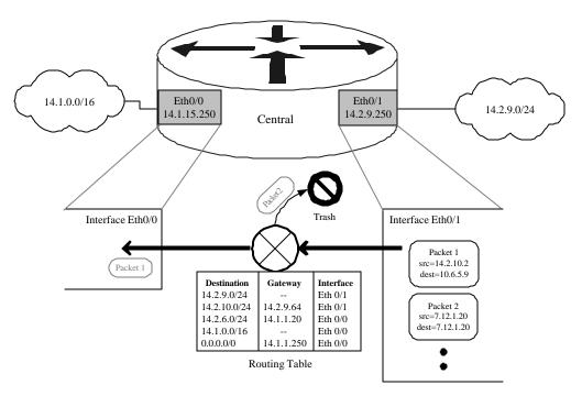
Figure 4-5: IP Unicast RPF Verification
