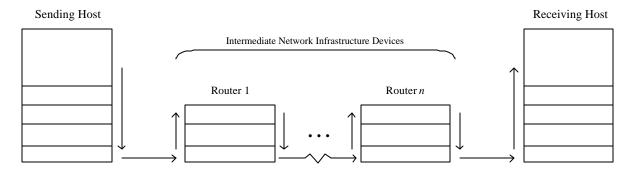
Figure 2-2: Moving Data through Protocol Stacks
