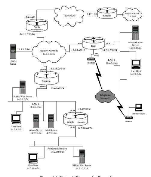
Figure 4-1: Network Diagram for Examples
