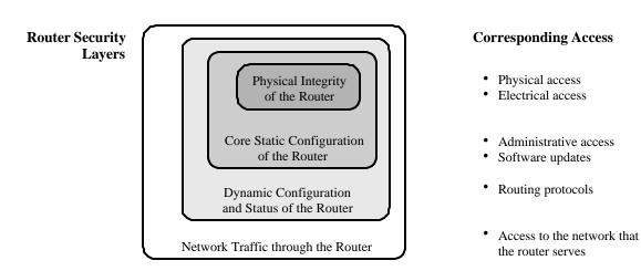
Figure 3-4: Layered View of Router Security
