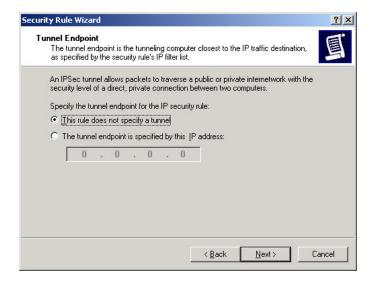
Since we selected transport mode when configuring the Cisco router, we do not need this tunnel. Continue on without specifying a tunnel. The next screen is about which network connections to use.
