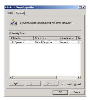
Two things must be done in this window. A new rule must be added, for which we will use the Add Wizard, which we will do in a second, but before that, we will configure the key exchange parameters (which were called by the name isakmp in the
