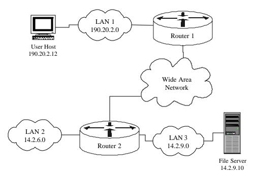
Figure 1-1 – A Simple Network with Two Routers
