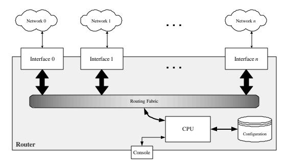
Figure 2-4: A Notional Router's Hardware
