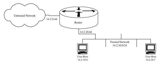
Figure 5-1: A Simple Router Firewall
