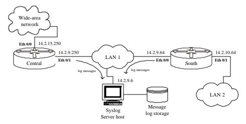
Figure 4-7: A Small Syslog Configuration
