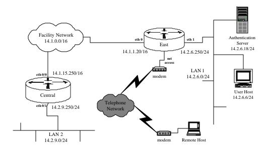
Figure 4-10: Router East in the Network
