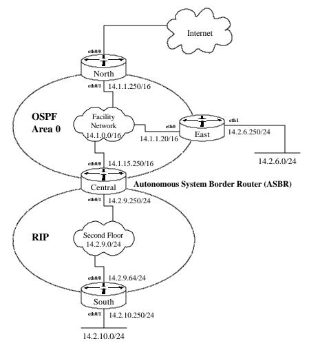
Figure 4-3: A Simple OSPF Routing Architecture
