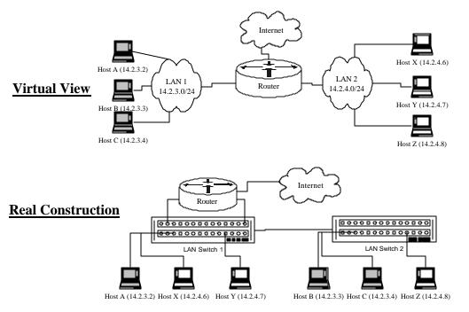
Figure 7-1: Virtual LAN Switching
