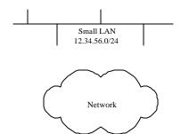
A local-area network (LAN) segment, such as an Ethernet, is represented by a horizontal or vertical bus, with several connections.
